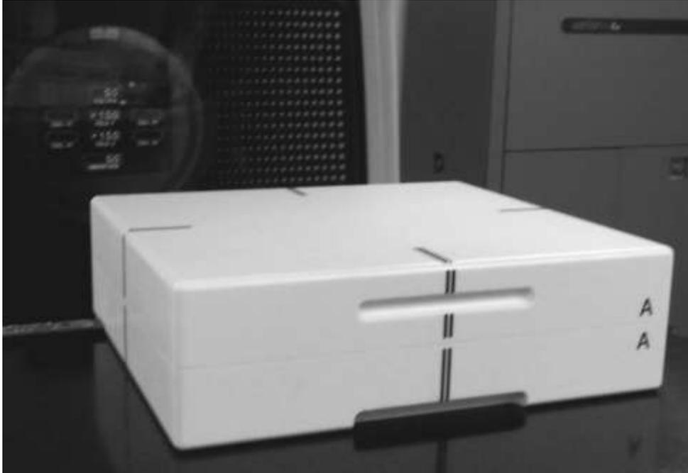
Figure 8: Finished setup of the GafChromic QuiCk Phantom™ on treatment couch
