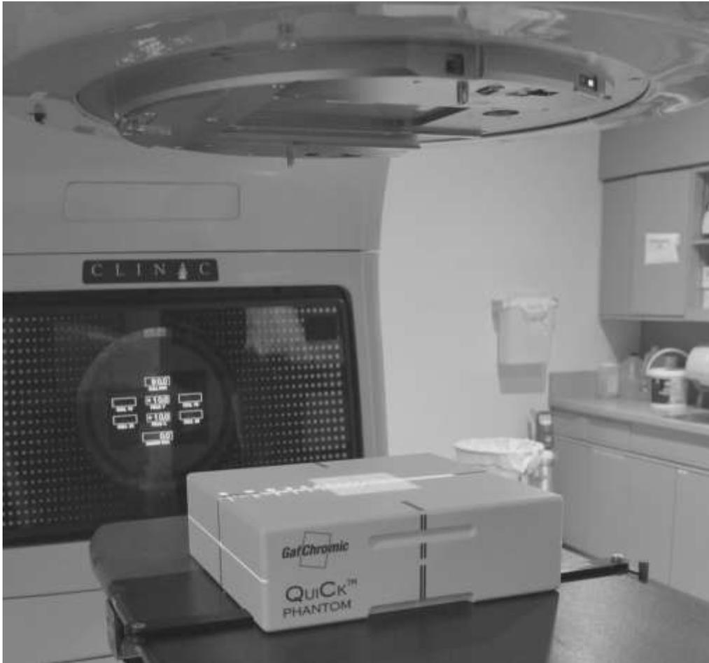
Figure 10: Isocenter alignment of phantom and radiation field
